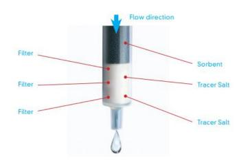
Patented environmental sampling method, SorbiCell, efficiently monitors water quality and enables tracing of hazardous chemicals in wastewater to their source, including hydrocarbons, chlorinated solvents, pesticides and heavy metals
