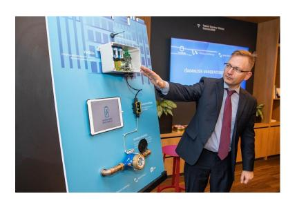
Smart water metering system using NB-IoT technology
